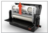
To replace, flip up the 5" adapter in the bottom center of the machine. Ensure the label on the refill cartridge is facing you, drop the cartridge into the machine using the track as a guide.
